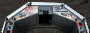
CONTROL PANEL Controls are duplicated on both sides of the cabin for ease of operation on either side of the ditch.
