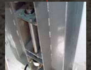
SPILL PAN VIBRATOR Prevents material from sticking to pan, especially when soil conditions are wet.
