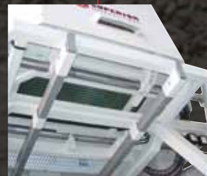
OSCILLATING CABIN Hydraulically slides out to either side of the machine to facilitate working on either side of the ditch.
