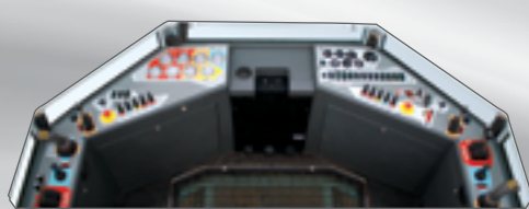
Control Panel The controls are duplicated on both sides of the cabin for ease of operation on either side of the ditch.
