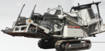
Adjustable Front/Rear Sections The front and rear can be adjusted hydraulically to compensate for different terrain gradients.
