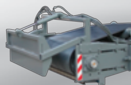
Adjustable Conveyor Dowel Controlled hydraulically to adjust angle and distance at which the material is placed back into the ditch.
