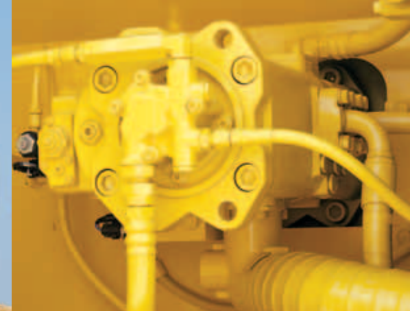
The hydraulic feed to the main pumps is positioned to draw fluid from the side of the hydraulic tank - rather than the tank bottom like many competitors. The hydraulic system utilizes a high capacity, small particle filtration system to provide industry leading maintenance intervals.
