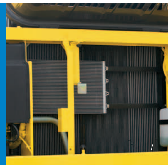
Side-by-side radiator, oil cooler and intercooler can be accessed easily for inspection and cleaning. The systems are separate, allowing the radiator to be removed for service without the need to drain the hydraulic system.
